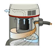
Due to the twist of the intake nozzle, the sprayfog is consequently diverted along the inner container wall. Additional filters are no longer necessary. The reliable floater system even reacts during heavy foam growth. Cooling air slots located on the side ensure the consistent separation of cooling and processed air.
