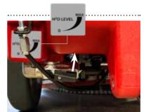
The water quantity can be adjusted for any floor covering.
