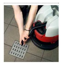
The dirty water tank can be emptied via the drain hose.
