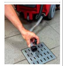
The clean water tank can be fully drained.
