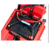
The maintenance-free gel batteries can be removed without tools via quick-connect couplings.
