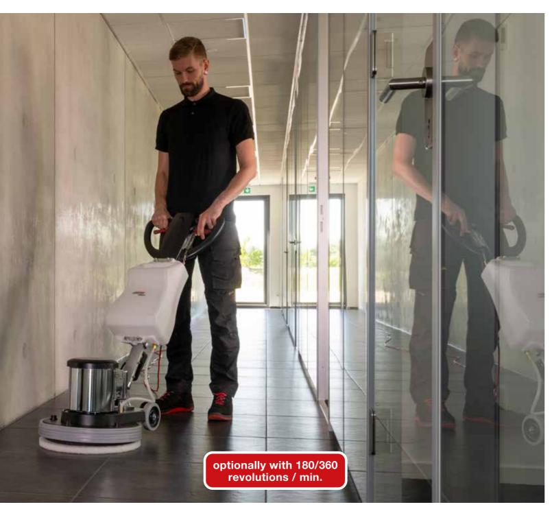
The Hercules Duo Speed combines the advantages of a slow and fast runner in only one device. Owing to its two working speeds, it is the perfect solution for efficient, fast an cost-effective cleaning and polishing.
