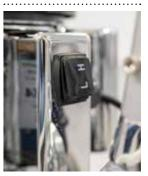
Switch to change operating speeds. L = 180 revolutions / min.
