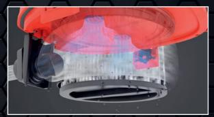
It consists of two independent filter chambers, which are cleaned one after the other. Suction current and suction power thus remain at a consistently high level even during cleaning, which guarantees permanent suction.
